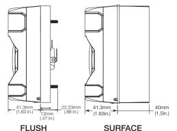
Drill out the (4) mounting holes, one in each corner using 5/32in. drill bit î up î Back box must be mounted with arrows pointing up
