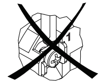
INCORRECT METHOD OF INSERTING MULTIPLE LEADS (BOTH WIRES ONE SIDE OF SCREW)
