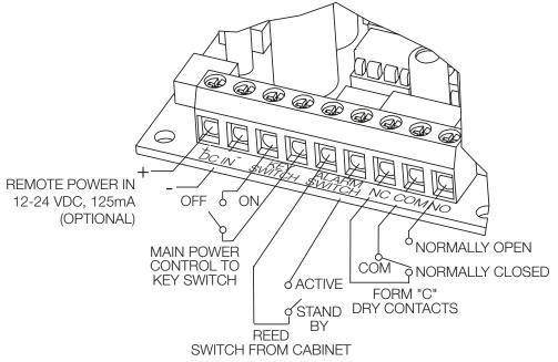
**Note** "DC IN" are the only polarity sensitive terminals.
