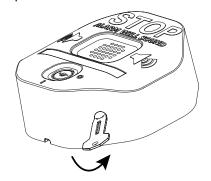
**3.** Remove cover from base, push on lock to separate
