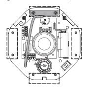
10. Position base. Mark and drill four (4) holes 1" (25mm) deep. Using plastic anchor, drill 3/16" (4.5mm). Install into wood or steel: drill 9/64" (3.5mm). Mount using (4) M4 x 25mm screws.
